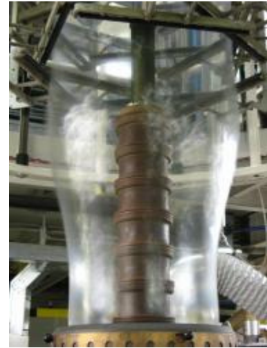
LyondellBasell's new grade, Adflex 7492 XCP , offers customers in blown film applications an outstanding combination of transparency and superior resistance to impact, puncture and tear propagation. With a film thickness of 30µm and 13 % haze value, the resin represents a new benchmark for highly-modified polypropylene grades
